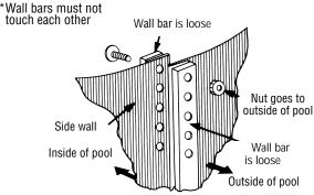
The Wall Bar is loose. It must be used when the wall is assembled on the job site as per drawings. Failure to do so will result in wall failure and voids the warranty
