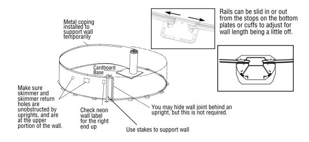
We manufacture two different kinds of wall joint assemblies. One has a single row of bolts and the other is a staggered double row pattern. In each case, the aluminum wall bars are not pre-attached. Please check which design your pool has and follow the appropriate instructions below.
