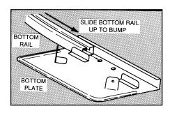
\* Adjust rails in or out as necessary to form a true circle. Please note the different bottom tracks.
