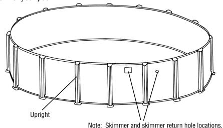
\*Wall joint is hidden behind the upright on most pools. This assures that the skimmer and the skimmer return holes are not obstructed. It is not possible to hide the wall bars on some of the smaller size pools that we make, such as the 12' round, and the 8' round.
